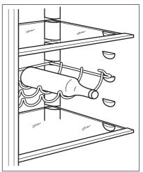
This shelf can be tilted to store unsealed bottles. To obtain this result, place front hooks of the shelf one level higher than the rear hooks.
