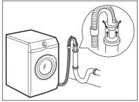
**i** The end of the drain hose must always be ventilated, i.e. the inner diameter of the drain pipe (min. 38 mm min. 1.5") must be larger than the external diameter of
