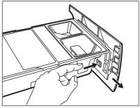
9. Make sure that all detergent residue is removed from the upper and lower part of the recess. Use a small brush to clean the recess.
