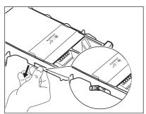
Press the catch on the back as indicated in the picture and lift up the top cover to remove it.
