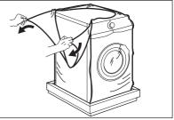
Open the door and remove the polystyrene piece from the door seal and all the items from the drum.
