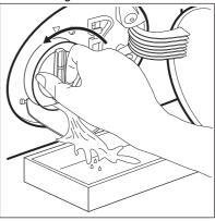
5. When the bowl is full of water, turn the filter back and empty the container.
