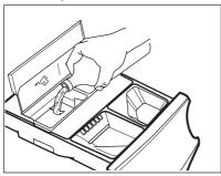
Gently pour only liquid softener in the AutoDose fabric softener tank <sup>(B)</sup>. Fill up to the maximum indicated level MAX
