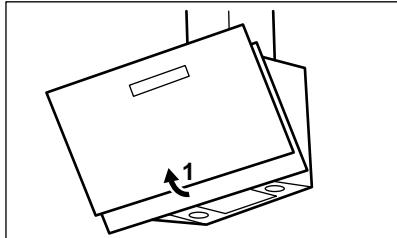
2. Press the handle of the mounting clip on the filter panel underneath the hood (1).
