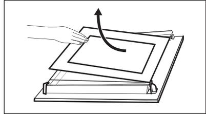
8. Clean the glass panels with water and soap. Dry the glass panels carefully. Do not clean the glass panels in the dishwasher. When the cleaning is completed, install the glass panels and the oven door.
